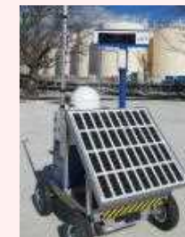
Installation of Dose-rate monitor
